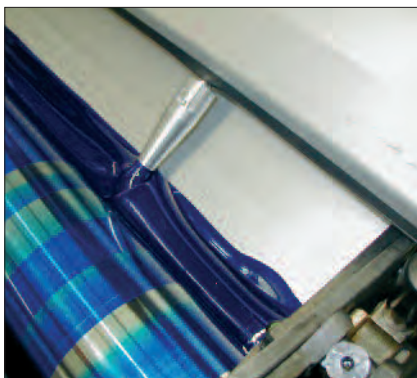
Ink agitators are recommended for UV ink which tends to stiffen and settle in the ink fountain. Source: MAN Roland.
