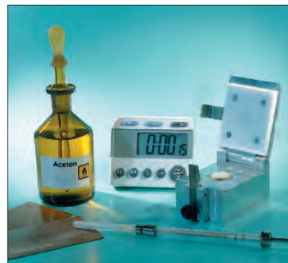
ACET is a simple to use solvent resistance test device developed by FOGRA. Source: FOGRA.
