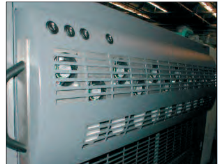
A blowing device combined with ink mist extraction. Source: MAN Roland.
