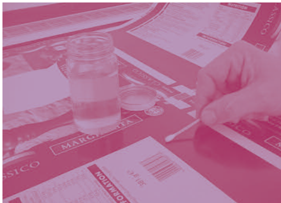
The traditional method to test if printed sheets have been adequately cured compares resistance to solvent attack between a printed sample and a standard test sample. Source: Sun Chemical.
